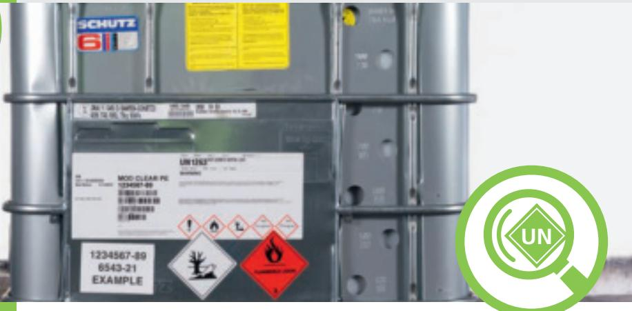
Label plates, product labels and hazardous material labels must be **legible**. Empty, uncleansed IBCs must carry the same markings (UN No. and name of the hazardous substance) and warning labels as filled containers (see ADR/international transport law).
